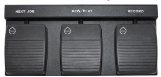
3 Press and hold down the "RECORD" pedal while speaking. If the Olympus DS-9500 Digital Recorder is in view (nearby), a small red light should light up during recording:
