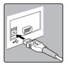
3 Make sure that the recorder is stopped, and then connect the USB cable to the connecting port on the bottom of this recorder.
