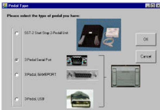
The first time you start the Start Stop application, it will show this pedal selection screen. Pick the type of pedal you have, then click OK and follow the on-screen directions. (If you make a mistake, or want to re-start this screen, click on “Configure”...”Select Pedal Type” from the Start Stop’s main screen.
