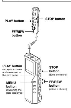
When the remote controller microphone is connected, buttons with the same names as those on the recorder work analogously.
