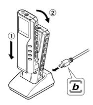
While pushing down the top of the recorder, set the recorder on the cradle. In this case, make sure that concavity on the rear of the recorder fits convexity of the cradle.
